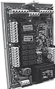
SIOS is a board equipped with 8 relays with potential free contact to control the activation or deactivation of remote electric utilities. Moreover, the board has 8 digital inlets to display the actuators or external consents, such as motor or other. The SIOS boards can be connected to a TODS panel (one SIOS for each TODS panel).
